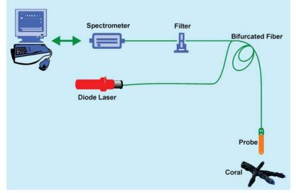
Fig. 1.3.4.1 Schematic diagram of the portable fiber optic fluorosensor
