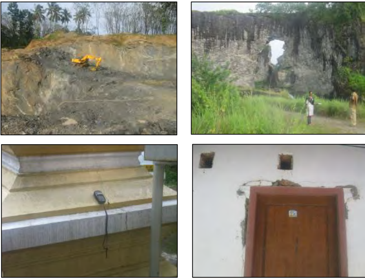
Fig. 4.2.2.1 Some selected scenes of hard rock quarrying and related environmental issues in the PRB: an active hard rock quarry (above left), an abandoned derelict site of past quarrying (above right), cracks and damages to structure due to vibration effects of blasting (below right & left)
