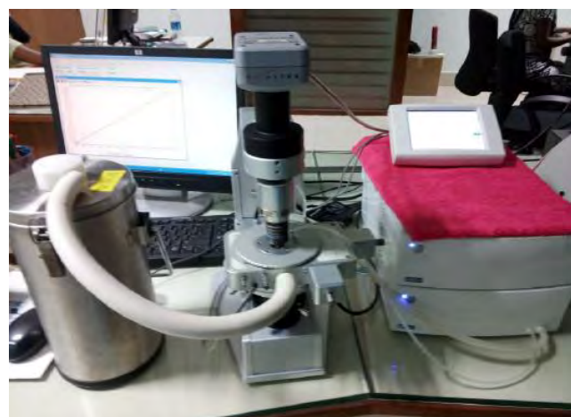
Fig. 1.7.2 Linkam heating freezing stage with imaging station for microthermometric studies of fluid inclusion
