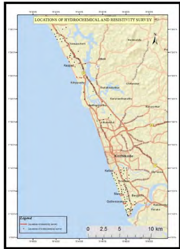
Fig. 2.8.5 locations of Hydrochemical and resistivity survey
