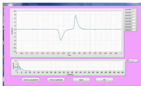
Fig. 3.1.4 Recorded the output from raindrop charge sensor using HFVR when a negatively charged raindrop passed through
