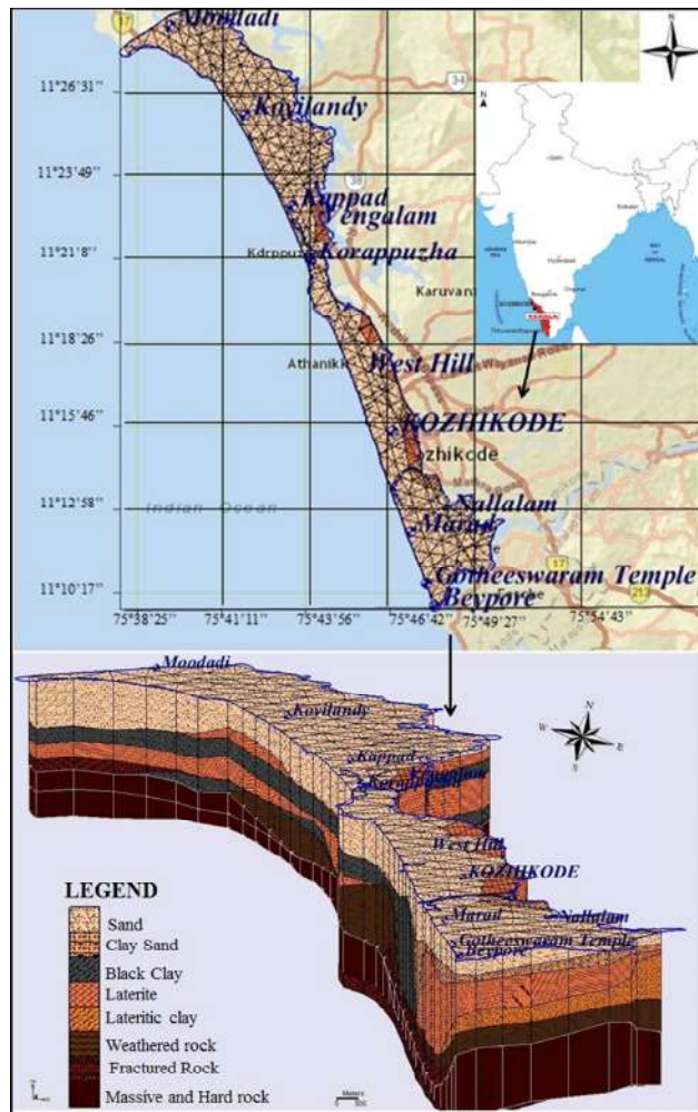
Fig. 2.8.1.1 Kozhikkode coastal aquifer and its lithology
